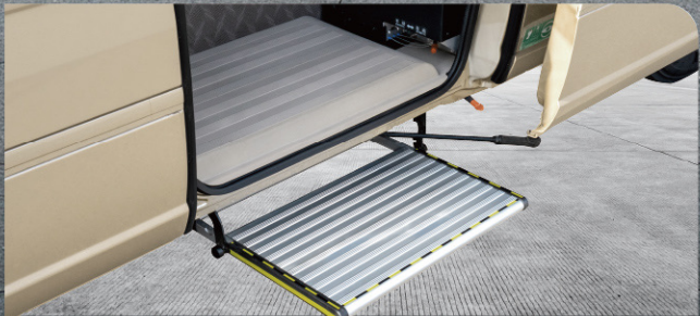
■ ELECTRIC STEP A movable step is configured as standard, with ground clearance of 190mm after extension, and heights of two steps are basically the same, achieving effortless boarding and alighting.
