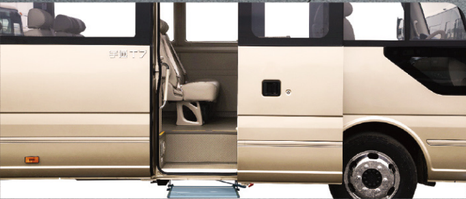
■ ELECTRIC OUTWARD SWING SELF-SUCTION DOOR A 740mm ultra-wide electric outward swing self-suction door is outfitted, which closes in 4-4.5 seconds.
