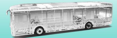
**Overall structure safety—vehicle body collision safety ensured:** designed into the diamond closed-loop structure, with key stress profile made of lightweight high-strength steel (the tensile strength reaches 750-880 Mpa), making the vehicle body stronger and safer.
