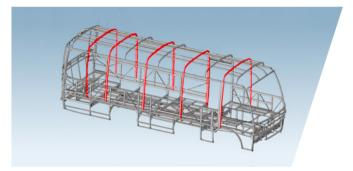
Diamond ring high-strength steel skeleton body is adopted, which is safer than stamped body. When the vehicle collides (whether frontal or side collision), the body deformation is small, which effectively protects the safety of drivers and passengers in the vehicle;
