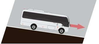
The retarder or exhaust brake auxiliary brake configuration improves long-slope braking safety and reduces brake pad wear in bus working conditions;
