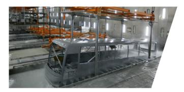
Yutong has the world's largest vehicle electrophoresis production line, equipment imported from Germany and more than 8 years of vehicle anti-corrosion commitment;
