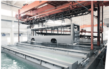
World leading bus body cathode electrophoresis Significantly improve corrosion resistance and durability, thereby boosting economic benefits throughout the product life cycle.
